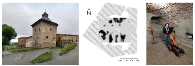
Figure 3: Pentagonal Tower of the Medzhybizh Fortress. Time slice from 1.83 m shows stone structures under the floor.
