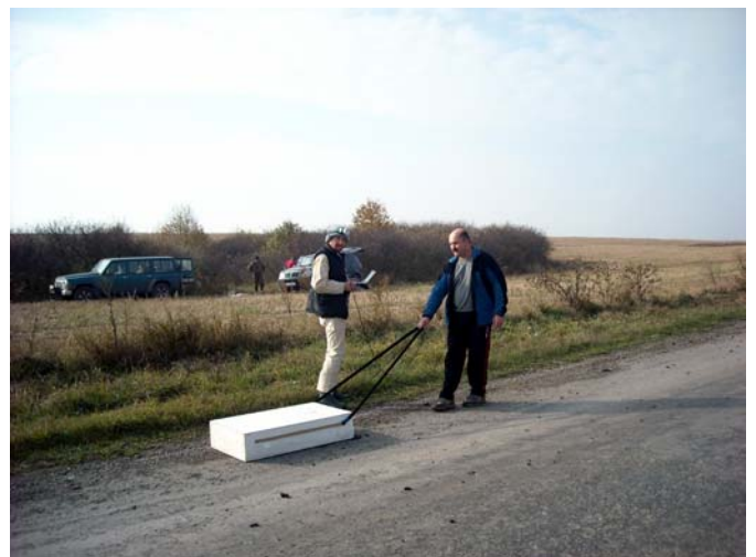
Figure 5. Subsurface data acquisition by VIY 2-125 GPR
